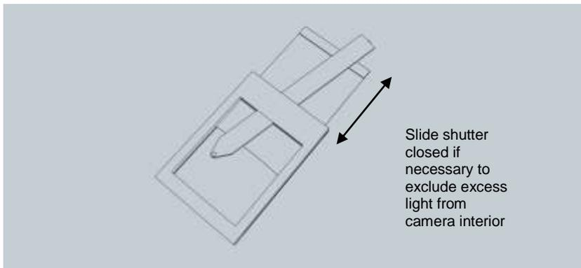
Insert the metering probe into the wider of the two slots in the top of the frame, if it is not already inserted. The sensor should be facing the front (lens) of the camera. If it is not clear which side is the sensor, the connector block at the other end of the probe should be on the front side. A white circle on the rear of the metering probe indicates the location of the sensor.
