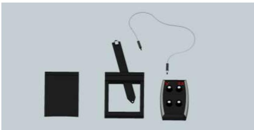
Insert 9V battery type - 6LR61 / 1604A / PP3. The battery compartment is on the rear of the case. The label inside the battery compartment indicates the polarity. The meter is designed with protection for reverse battery connection in case the battery is inadvertently inserted the wrong way round.
